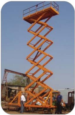
Towing Scissor Lift upto 16m & optional powered movement with capacity upto 1 ton.
