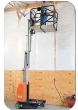
Aerial Working platform to accommodate one person for height reach upto 10m can be battery operated
